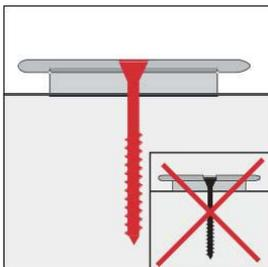
Please use the correct torque to ensure the screw head finishes level with the clip surface. Do not insert the screw too deep into the clip. This could damage the clip.
