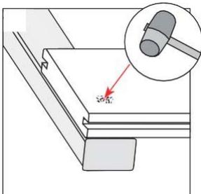
**Note!** The displaced decking material may be removed when washing the deck particularly with a high pressure washer.
